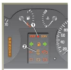
Warning light to indicate that the system is not operating correctly After the ignition has been switched on, if tell-tale light 1 continues to flash or remains steadily lit, this indicates that the system is not operating correctly.
