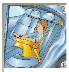
A booster seat with a height-adjustable seatback and a belt guide is recommended as this will allow the belt to be worn as close to the base of the neck as possible but not on it. A bucket-type seat (figure 4) must be used for vehicles where the rear centre seat is equipped with a two-point belt.
