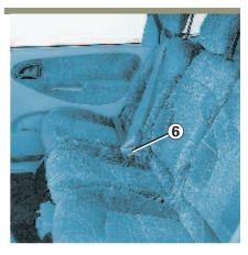
Lock the remaining sliding buckle  $\bf 5$  into the red catch  $\bf 6$ .
