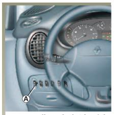
Button A allows the height of the beams to be adjusted in relation to the load.
