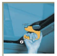
Lower handle **2** and rotate it through a quarter of a turn and push the lever back into position.
