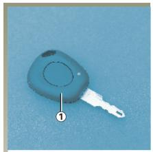
1 Radio frequency remote control locking unit, ignition key, key for doors, luggage compartment and fuel filler flap.
