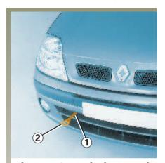
The steering wheel must be unlocked and the ignition key must be in position "M" (ignition "on") to provide stop lights and direction indicators on the towed car. The towed vehicle lights must be switched on at night.
