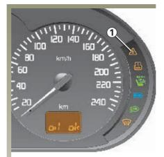
Disabling the traction control function also deactivates the ESP function: refer to the information on ESP in section 2.
